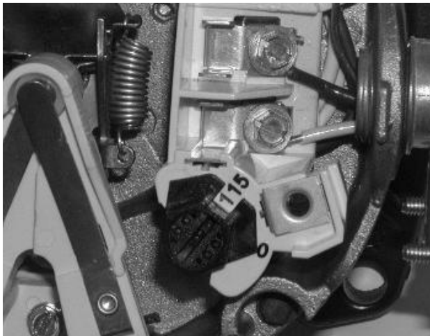
Figure 4: Motor Set for 115 Volt Operation
